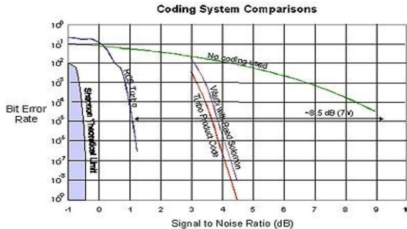
Fig 7 : Comparison of the SNR and BER of Coding system
