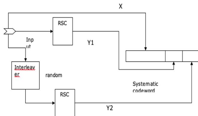
Fig 4: Coding Architecture
