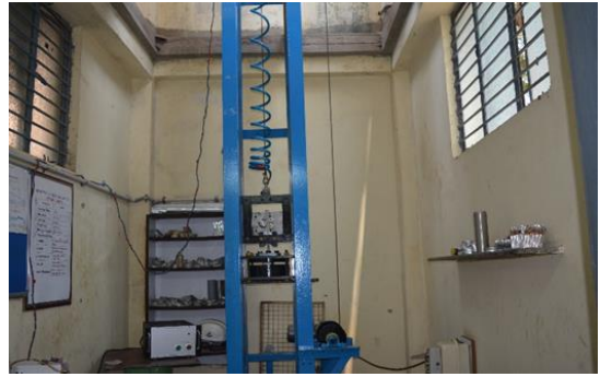
Automatic releasing mechanism for the drop weight test facility.
