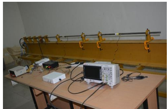
Split Hopkinson Pressure Bar (SHPB) Test Setup.
