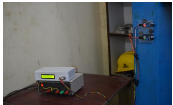
Velocity measurement device for drop weight impact test machine.
